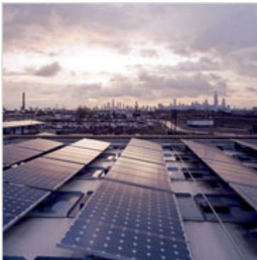
Photovoltaic systems on the roof and the south facade reduce the cooling load while generating power. A stormwater management system recharges groundwater, reduces outflow to the city's sewer system, and biologically cleans the parking lot runoff.
